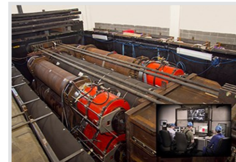
C-FER technicians utilizing automated instrumentation to remotely monitor loads, pressures, temperatures, displacements and strains on pipe specimen during testing.
