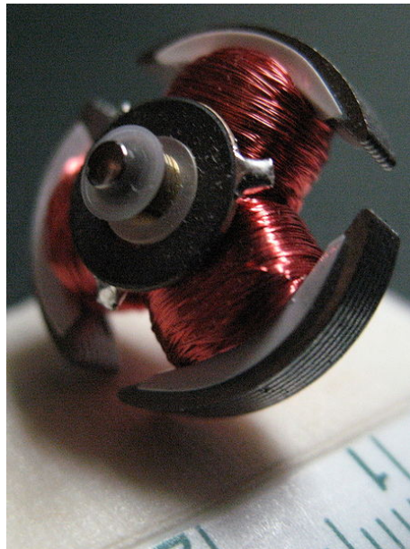
DC Motor -- Wired Rotor
